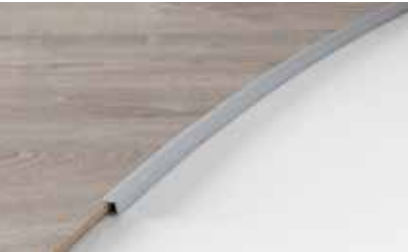
End profile, bendable NEBENDPCSILVME270, 2700 x 28 mm For finishing laminate “islands” in curved shapes. Height 13.1 mm. Surface: silver anodized aluminium. 10 pc / pack. To be installed with special bending tool NEBTOOL.
