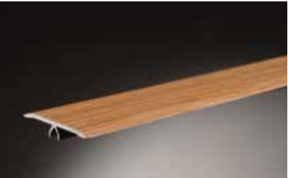
T-moulding, colour matched PGEXPC(-), 2350 x 50 mm (see matching matrix for correct art no) From laminate to laminate. Easy installation with snap-in function. Material: solid aluminium. Surface: flooring laminate, TitanX™-surface. Bottom part: galvanised iron. Minimum order quantity: 30 pc.
