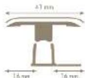
Saw the profile to the right length. Cut away section A and section B with the knife to make the expansion profile.
